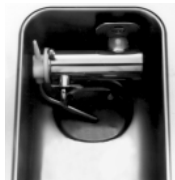
In-Hopper Air/Mix Pump
